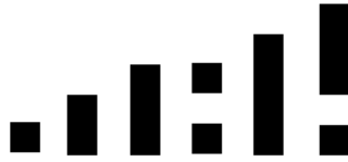
Fig. 4. Close-up on a bitmap generated after static mode tests and showing the shape of single word errors or small cluster of errors.
