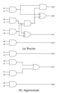
Fig. 1: Two-bit multiplier Example
