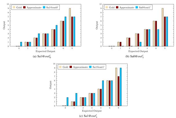
Fig. 4: Accuracy Degradation due to Fault Escape
