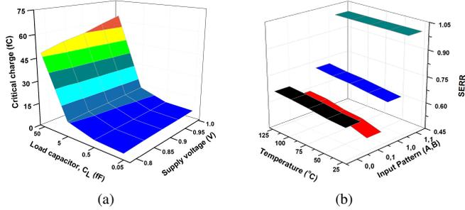
**Fig. 4:** (a) Two-input NAND gate critical charge characteristics shown at different supply voltages for various load capacitors ( $C_L$ ). (b) Soft error rate ratio (SERR) with stress time at various operating temperatures for all possible input combinations of two input NAND gate.
