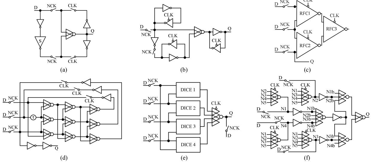
Fig. 2. Schematics of previous hardened latches. (a) DET-SEHPL [19]. (b) LSEH [20]. (c) DNURL [21]. (d) THLTCH [22]. (e) TNUDICE [6]. (f) TNUHL [5].
