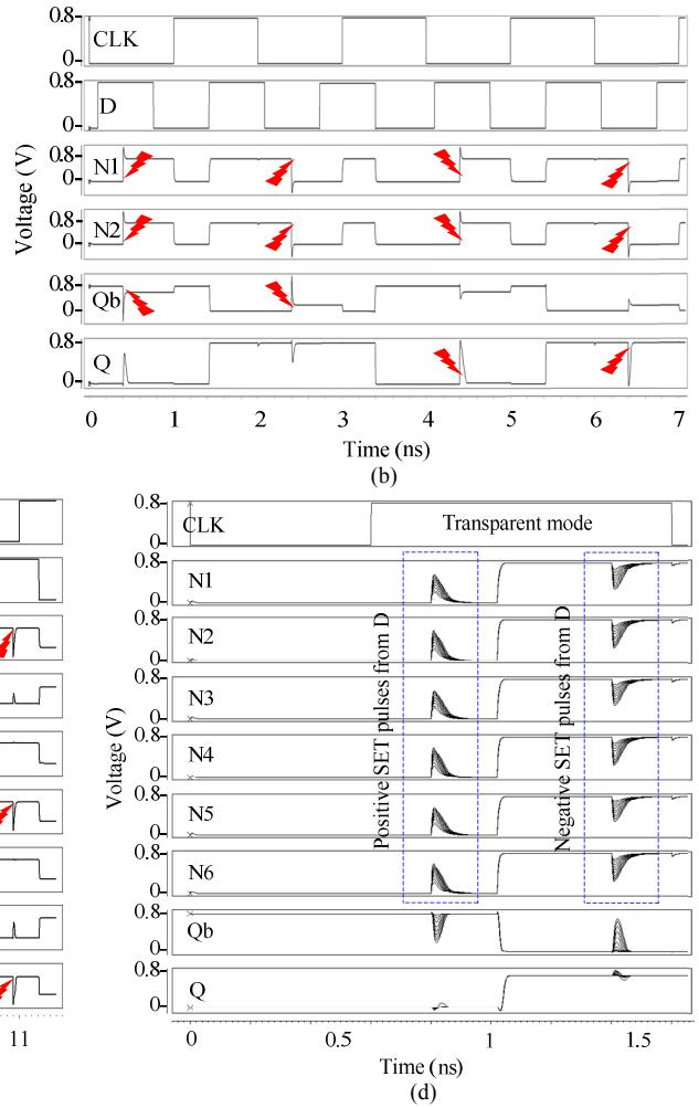
Fig. 4. Simulation results of the proposed HITTSL latch. (a) Key TNU injections for  $\langle N1, N1b, Qb \rangle$  and  $\langle N1, N1b, Q \rangle$  of Case T1. (b) Key TNU injections for  $\langle N1, N2, Qb \rangle$  and  $\langle N1, N2, Q \rangle$  of Case T1. (c) Other key TNU injections. (d) SET injections.
