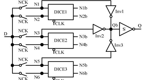
Fig. 3. Proposed HITSFL latch design.
