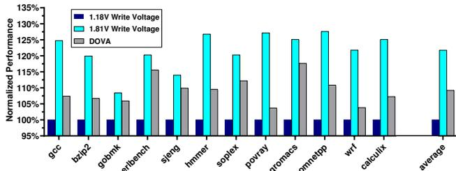
Fig. 6. Normalized performance improvements when running SPEC2K6 benchmarks on a quad-core processor.
