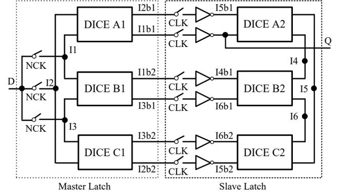
Fig. 2. Schematic of the proposed DURI-FF cell.
