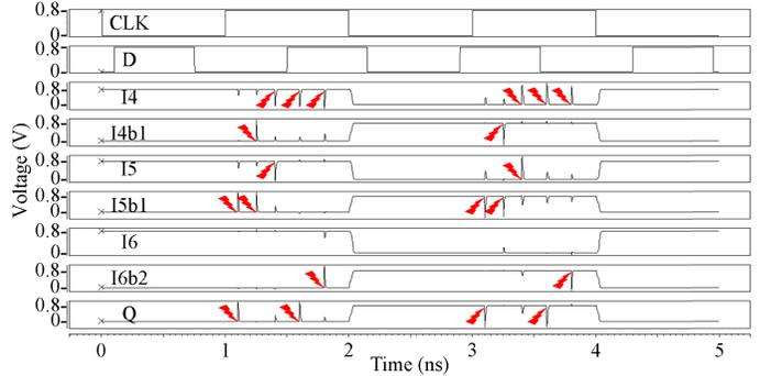
Fig. 4. Simulation results of all indicative DNU injections for the slave latch of the proposed DURIF-FF cell.
