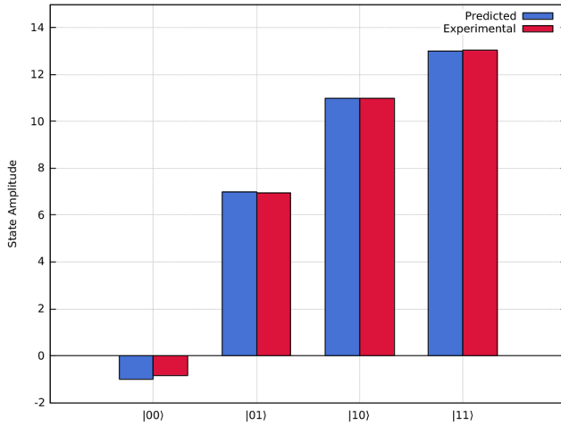
Fig. 5 Blue bars represent the predicted state amplitudes for the solution vector |x\rangle . The red bars indicate the simulated experiment results using Qiskit Aer QasmSimulator (a noisy quantum simulator backend) for the state amplitudes. The states have not been normalised, so that the deviation from the solution of the original linear equation system is prominent
