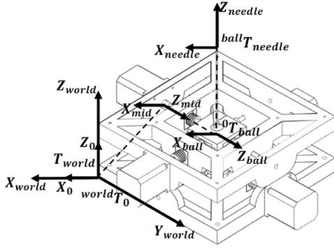
Fig. 5. Transfer matrix relationship of the robot.
