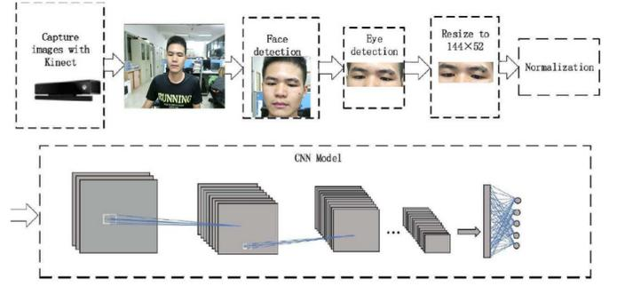
Fig. 7. Workflow of eye-gaze direction estimation algorithm.
