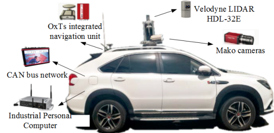
Fig. 3. BIT intelligent vehicle platform
