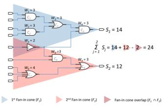
Figure 1. Application of the structural susceptibility analysis
