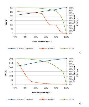
Figure 3. Scenario comparisions with respect to S1 with a) S2 for the add, b) S2 for the mult, c) S3 for the add and d) S3 for the mult
