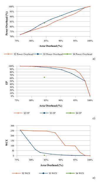
Figure 4. All scenario comparisions with respect to S1 with a) power overhead for the add, b) power overhead for the mult, c) EP for the add, d) EP for the mult, e) WCE for the add and f) WCE for the mult
