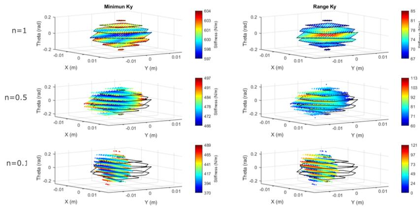
Fig. 6 The stiffness ranges  $K_y$  with  $n = 1, 0.5$  and  $0.1$
