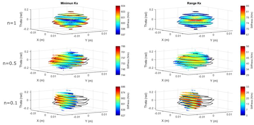
Fig. 5 The stiffness ranges  $K_x$   $n = 1, 0.5$  and  $0.1$
