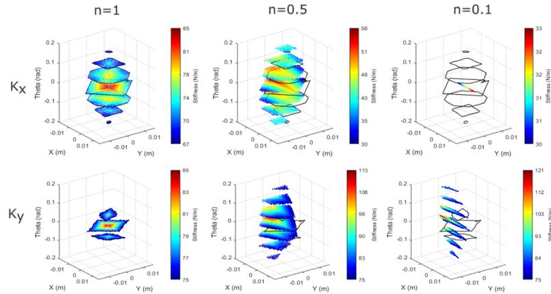
**Fig. 8** Workspace using  $K_x=30$  N/m and  $K_y=75$  N/m
