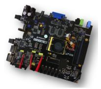
Figure 6: The Genesys FPGA board used for compute node prototype.
