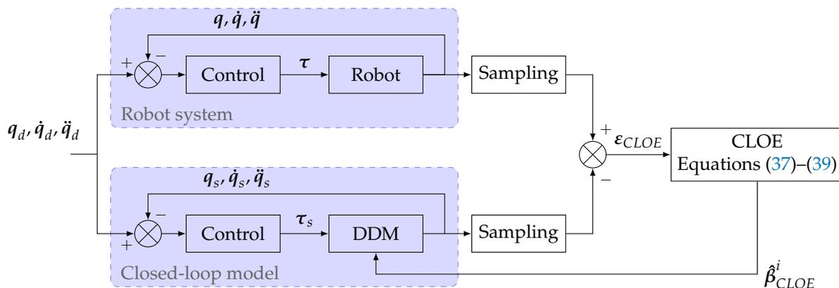
Figure 2. Block diagram of the CLOE identification method.
