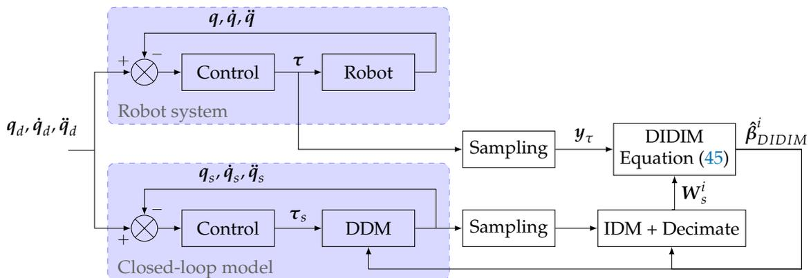
Figure 4. Block diagram of the DIDIM identification method.
