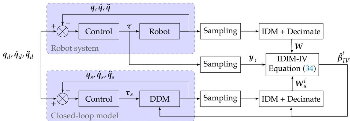
Figure 1. Block diagram of the IDIM-IV identification method.
