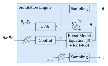
Figure 7. Detail of the "Simulation Engine" of Figure 6.
