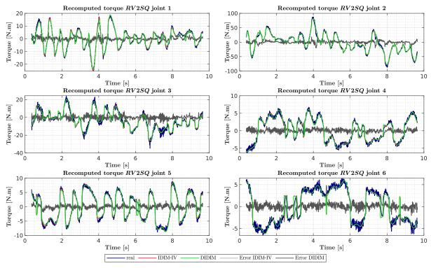
Figure 10. Reconstructed IDIM-IV and DIDIM torque signals during the validation experiment on the real RV2SQ robot.
