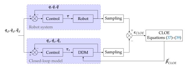
Figure 2. Block diagram of the CLOE identification method.
