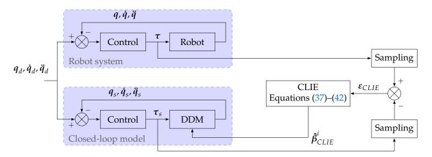
Figure 3. Block diagram of the Closed-Loop Input Error (CLIE) identification method.
