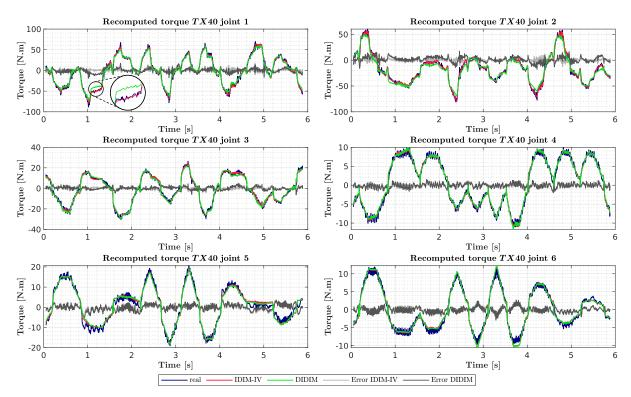
Figure 9. Reconstructed IDIM-IV and DIDIM torque signals during the validation experiment on the real TX40 robot.
