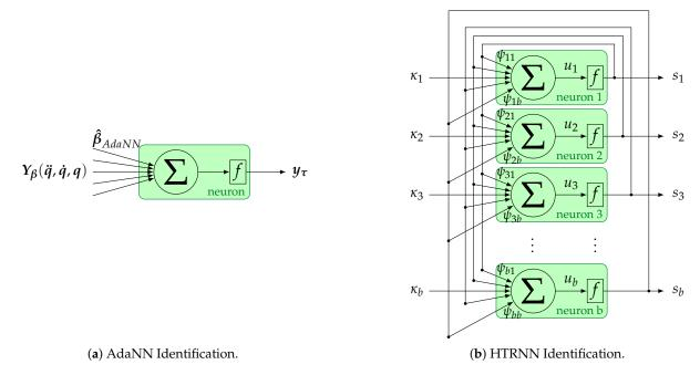
Figure 5. Adaline and Hopfield Neural Networks used for Inertial Parameter Identification.
