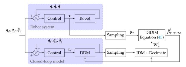
Figure 4. Block diagram of the DIDIM identification method.
