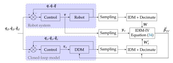
Figure 1. Block diagram of the IDIM-IV identification method.
