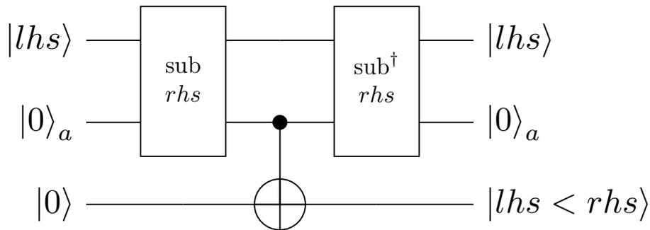
FIG. 12. Computation of the high-bit of  $lhs - rhs$  with a  $(n + 1)$ -qubit subtractor. The second quantum register is an ancilla qubit that is appended to the quantum register storing  $|lhs\rangle$  in order to form a  $(n + 1)$ -qubit register. The result is stored in a third quantum register as  $|1\rangle$  if  $lhs < rhs$ , else  $|0\rangle$ .
