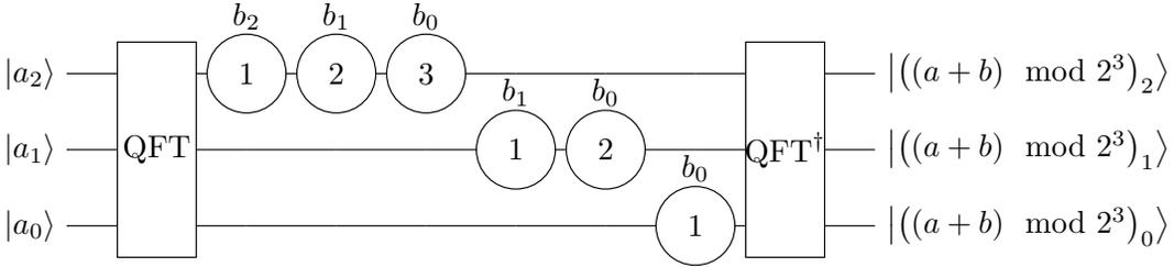
FIG. 11. Modified Draper’s adder example for 3-qubit register  $|a\rangle$  and 3-bit classical constant  $b$ . The round gates between the two applications of the Quantum Fourier Transform (QFT gates) are phase gates and are defined in [34]. A label  $b_i$  above a phase gate means that the phase gate should only be applied when the  $i^{\text{th}}$  bit of  $b$  is set to 1. Note that the adder wraps on overflow, meaning that if an overflow happens, the result will be  $(a + b) \bmod 2^3$ .
