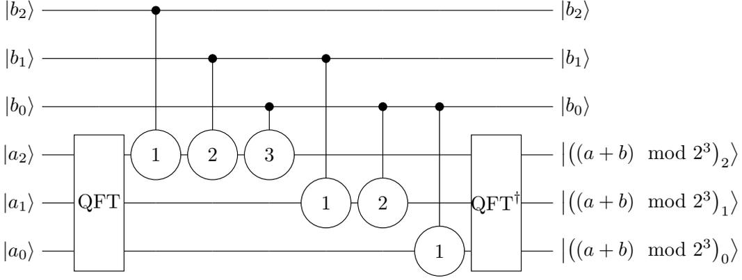
FIG. 10. Original Draper’s adder example for 3-qubit registers  $|a\rangle$  and  $|b\rangle$ . The round gates between the two applications of the Quantum Fourier Transform (QFT gates) are controlled phase gates and are defined in [34]. Note that the adder wraps on overflow, meaning that if an overflow happens, the result will be  $(a + b) \bmod 2^3$ .
