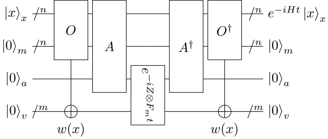
FIG. 7. Quantum circuit re-created from [10, p. 71] that simulates a 1-sparse integer-weighted Hamiltonian for a given time  $t$ .  $O$  is the implementation of the oracle,  $A$  is a quantum circuit defined in [10, p. 70].  $F_m$  is defined as the diagonal matrix with diagonal entries increasing from 0 to  $2^m - 1$  (see eq. (C7)).
