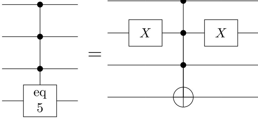
FIG. 13. Example of **eq** gate implementation for the compile-time value 5. **X** gates are applied to the second control qubit because the only bit set to 0 in the big-endian binary representation of  $5 = 101_2$  is at the second (middle) position.
