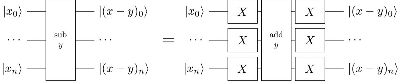
FIG. 9. Implementation of the **sub** gate from an **add** gate. The  $y$  value encoding is intentionally omitted. The subtractor will use the same encoding as the adder (i.e. either the  $y$  value is encoded on a quantum register or it is encoded directly in the quantum circuit implementing the adder). Note that the  $y$  value is not negated.
