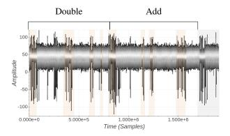
Figure 8: *Rhea* EM Trace - ECDSA Signature (P-256, SHA-256) - Scalar Multiplication Single Iteration
