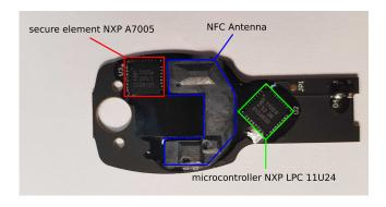
Figure 2: Google Titan Security Key PCB, with annotated main parts
