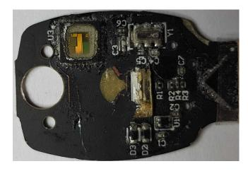
Figure 3: *Google Titan Security Key* PCB, with NXP A7005a die visible after wet chemical attack of its package
