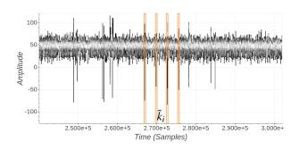
Figure 10: *Rhea* EM Trace - ECDSA Signature (P-256, SHA-256) - Sensitive Leakage
