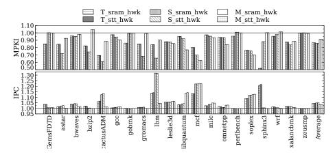
Fig. 9. Performance impact of Hawkeye normalized to LRU for a monocore
