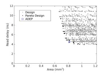
Fig. 5. Pareto view of all cache configurations for read delay according to cache area
