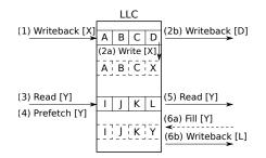
Fig. 2. Write transactions on the Last-Level Cache
