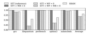
(a) Write-back (WB) and write-fill (WF) effects on performances normalized to baseline STT-MRAM
