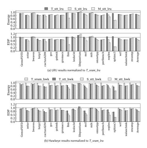
Fig. 10. Energy consumption (top) and EDP (bottom) for a monocore platform with LRU and Hawkeye replacement policies
