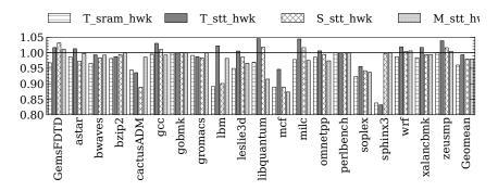
Fig. 12. Energy impact of the Hawkeye replacement policy on a monocore platform. For each configuration with Hawkeye, result is normalized to its counterpart with LRU.
