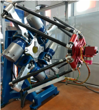
Fig. 2. View of SPIDER4 parallel robot used for real-time experiments.
