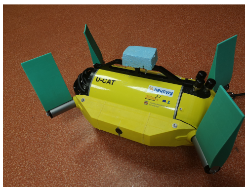
Figure 14: U-CAT pictured with an added buoyancy foam fixed on its top.
