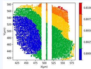
Supply voltage of the library assigned to each standard cell for first iteration
