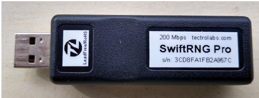
Figure 6.8: Tectrolabs Swift RNG, PRO version
