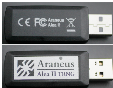
Figure 6.3: Araneus Alea II True Random Number Generator (both sides). The LED is visible near letter “e” in “Araneus”.
