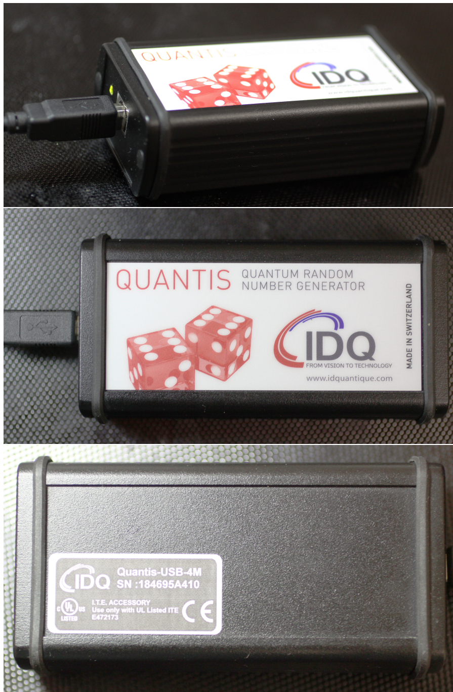
Figure 6.12: Random number generator from IDQuantique, USB version
