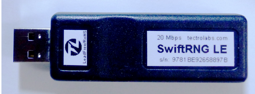
Figure 6.5: Tectrolabs Swift RNG, LE version
