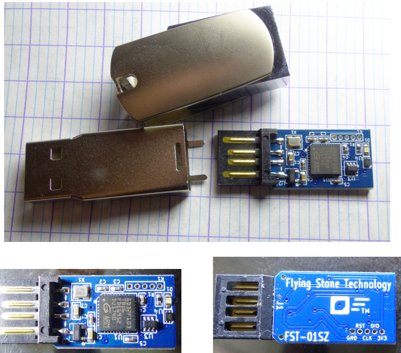
Figure 6.4: Gniibe random number generator, a firmware for FST-01SZ (both sides)
