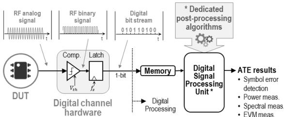
Fig. 4. Proposed digital approach for testing ZigBee devices.
