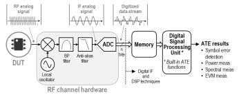
Fig. 2. Current industrial setup for testing ZigBee devices.
