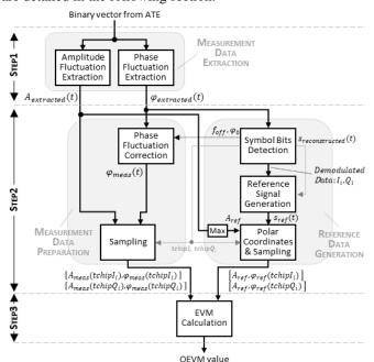
Fig. 5. Block diagram of the post-processing algorithm for EVM measurement.
