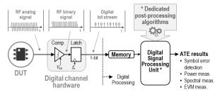
Fig. 4. Proposed digital approach for testing ZigBee devices.
