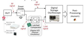
Fig. 15. Experimental setup for lab experiments.
