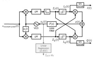
Fig. 12. Costas loop for demodulation of OQPSK signals with pulse shaping.
