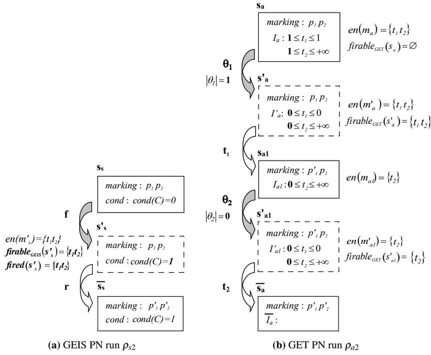
**Fig. 12** Equivalent runs with two simultaneously fired transitions
