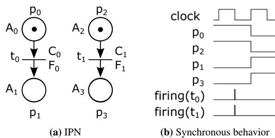
Fig. 3 Simultaneous firing of transitions in synchronous execution
