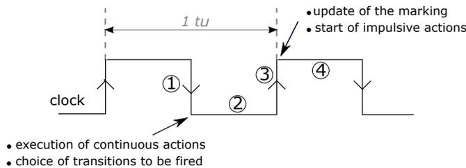
Fig. 2 Principle of the synchronous implementation of IPN
