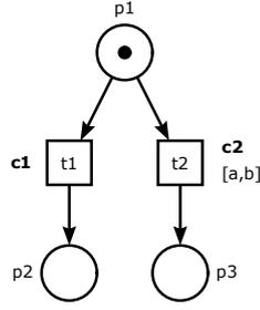
Fig. 16 Example of a potential blocking situation
