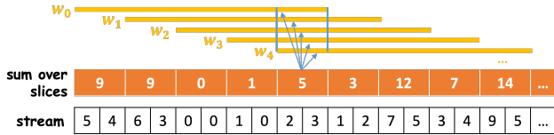
Figure 1: Example of computing sum over a count-based sliding window with a range of 10 values and a slide of 2 values.
