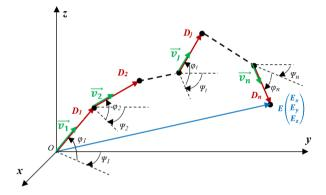
Figure 1: Parametrization of the kinematic chain.
