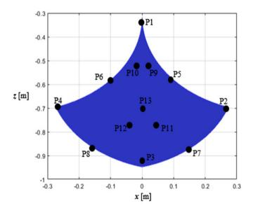
**Figure 13**: The Pi points in the W workspace of the PAR2 PKM.
