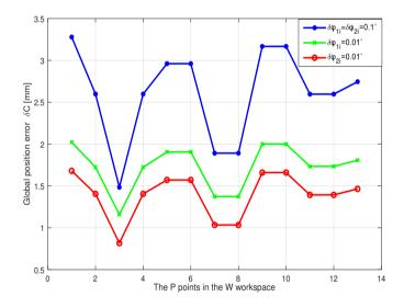
Figure 11: Variation of the position error as a function of the variation of angular errors.
