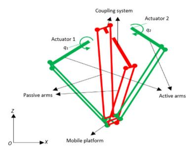
Figure 3: Schematic CAD view of the PAR2 PKM.
