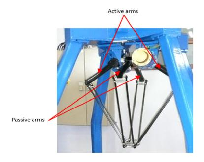
Figure 2: View of the PAR2 parallel manipulator [34].
