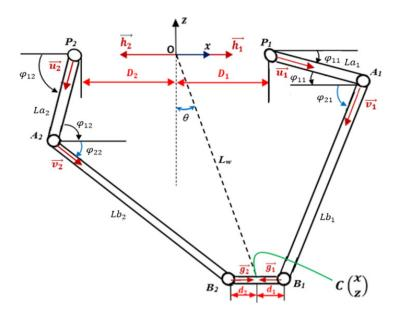
Figure 4: Parameterization of the PAR2 robot.
