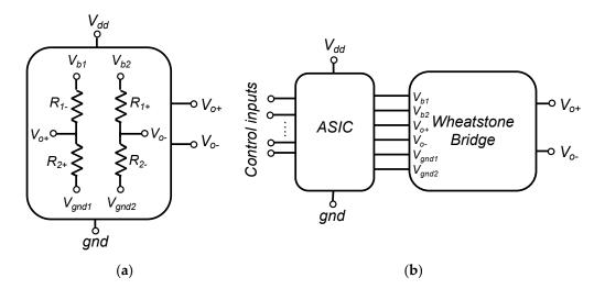
**Figure 1.** (a) Wheatstone bridge arrangement of a resistive sensor, (b) Wheatstone bridge connection to the « soft » trimming ASIC.
