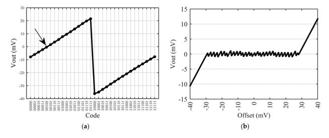
**Figure 14.** Measured output voltage of the smart-trimmed sensor after coarse tuning: (a) sensor output voltage vs. 5-bits code with arrow representing optimal code for this example, (b) sensor output voltage vs. initial offset.
