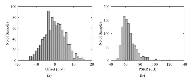
**Figure 2.** Impact of resistance mismatches on two performances of a Wheatstone bridge: (a) Offset in mV and, (b) power supply rejection ratio measured at 1 kHz in dB.
