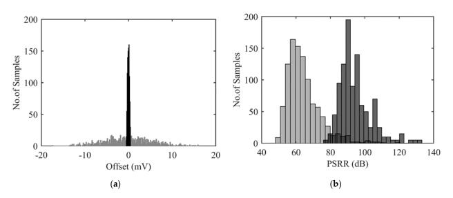
**Figure 9.** Monte Carlo simulations: Offset (**a**) and PSRR (**b**) are reported for a WB before (in grey) and after (in black) offset compensation.
