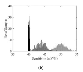
**Figure 11.** Results after scale factor adjustment: (a) variation of sensitivity (continuous line) and common mode voltage (dashed line) with Rgnd and  $R_{Vdd}$ , (b) Monte Carlo simulation of sensitivity of a bare Wheatstone bridge (light grey), an offset compensated Wheatstone bridge (dark grey) and a fully compensated Wheatstone bridge (in black).
