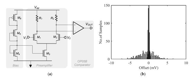
**Figure 8.** (a) A simple design to reduce offset of an existing comparator, (b) Monte Carlo simulations of input-referred offset of comparator IP (in grey) and a pre-amplified comparator (in black).
