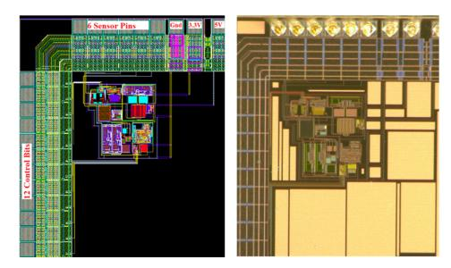
**Figure 12.** First demonstration IC for post-fabrication electrical trimming of resistive sensors: layout view (**left**) and photograph (**right**).
