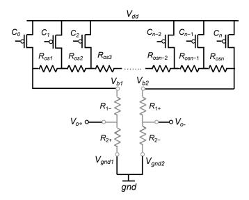
Figure 3. Basic architecture for offset compensation.
