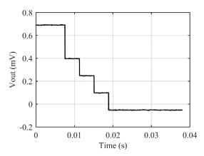
**Figure 16.** Auto zero procedure starts automatically at power-up to cancel-out most of the residual offset.
