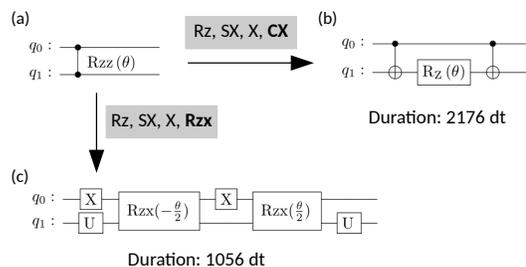
FIG. 1: (a) Original  $R_{ZZ}$  gate with  $\theta = \frac{\pi}{3}$ . The circuit is mapped to the first two qubits of IBM Q 27 Toronto. (b) The transpilation result with basis gate sets  $\{R_Z, SX, X, CX\}$ , and the duration is 2176 dt. (c) The transpilation result with basis gate sets  $\{R_Z, SX, X, R_{ZX}\}$ , and the duration is 1025 dt. We replace  $R_Z(\frac{m\pi}{2})\sqrt{X}R_Z(\frac{n\pi}{2})$  by  $U$  to simplify the circuit.
