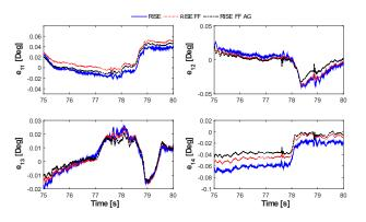
Fig. 11. Zoomed views of evolution of tracking errors versus time in joint space at low forward speed.
