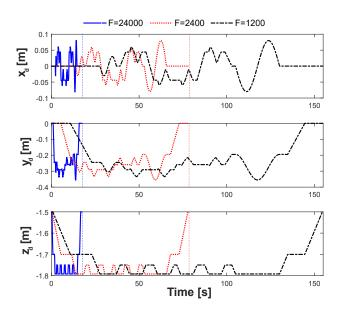
Fig. 8. Evolution of desired Cartesian trajectories versus time for different forward speeds F.
