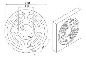
Fig. 6. Illustration of desired piece to be machined with its dimensions in mm and degrees.
