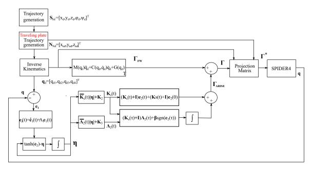
Fig. 3. Block diagram of the proposed control solution for SPIDER4 RA-PKM.
