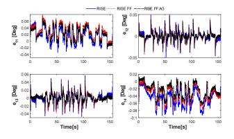
Fig. 10. Evolution of tracking errors versus time in joint space at low forward speed.
