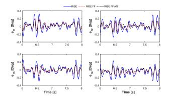
Fig. 21. Zoomed views of evolution of tracking errors in joint space at high forward speed.
