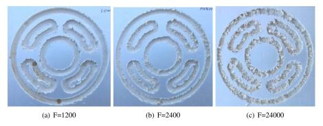
Fig. 25. View of the machining results using the proposed RISE FF AG controller with different Forward speeds (low, medium and high respectively).
