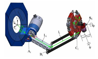
Fig. 2. Illustration of one kinematic chain of SPIDER4 RA-PKM.
