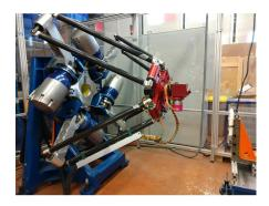
Fig. 4. Side view of experimental setup of SPIDER4 RA-PKM.
