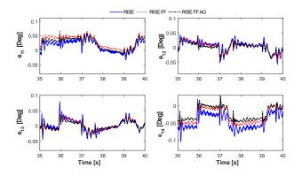
Fig. 16. Zoomed view of evolution versus time of tracking errors in joint space at medium forward speed.
