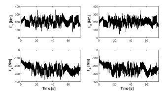
Fig. 19. Evolution versus time of control inputs generated by proposed RISE FF AG controller at medium forward speed.
