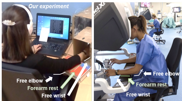
Figure 5. Left: forearm resting position in our experimental setup. Right: example of forearm resting position during robotic-assisted surgery training.
