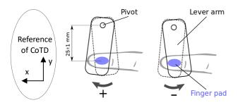
Figure 3. Scheme for one tactile actuator or tactor. The 2 directions of movement describing a short semicircular arc. For clarity, the rubber interphase is not shown, but it is the contact interface with the *finger pad*. The center of the region of the skin surface in contact with the tactor is called center of tangential displacement (CoTD).
