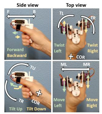
Figure 4. Different views of the portable HG device in the thumbindex grip configuration. The 4 pictures illustrate the 4-DoF of the induced hand movements shown by the white arrows, and the center of rotation (COR). The small arrows (green and yellow) indicate the STS on the *finger pads* of the pair of fingers. The arrow size indicates the movement magnitude. A video describing the device is included as supplementary material and available <u>here</u>.
