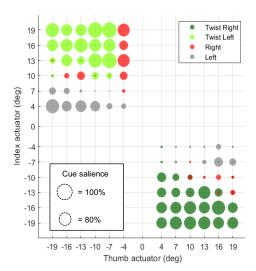
**Figure 6.** Hand *movement cues* identified in Test 1a. Participants used the thumb-index finger pair to grab the device. They were obliged to choose between 2-DoF and the "unclear" feeling.
