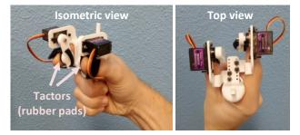
**Figure 2.** Different views of the portable HG device in the thumbindex grip style. Views show the lever arms of each servomotor that jointly perform STS on the thumb and index *finger pads*. The top view better depicts the adjustable position of the actuators on the handle to adapt the device to users with different hand sizes.
