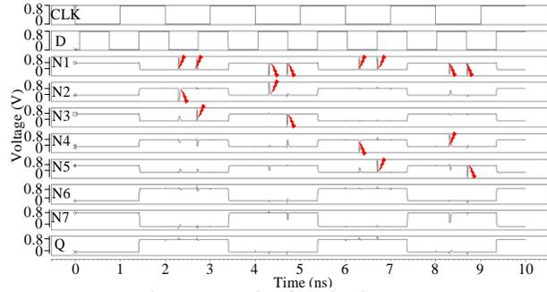
**Figure 5: Simulation results for the key DNU injections for <I1, I2>, <I1, I3>, <I1, I4>, and <I1, I5> of the proposed HRLD latch (Note that any single node can be set as the output of the latch so that any node pair comprising Q is also DNU recoverable and this is also true for cases in figure 6).**
