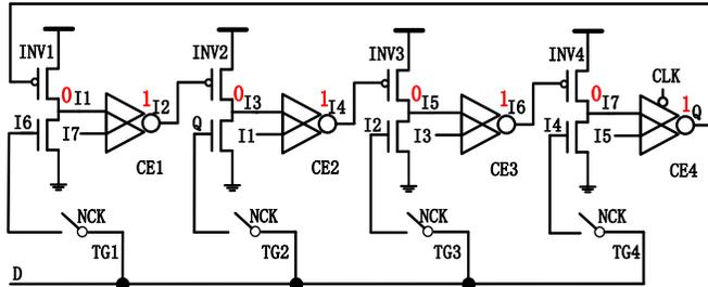
Figure 2: Schematic of the proposed HRLD latch.
