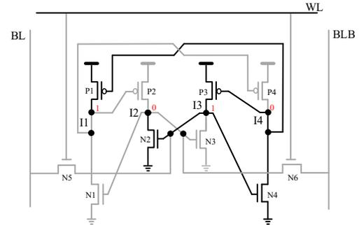
Fig. 1. Schematic of the proposed RHBD10T cell.
