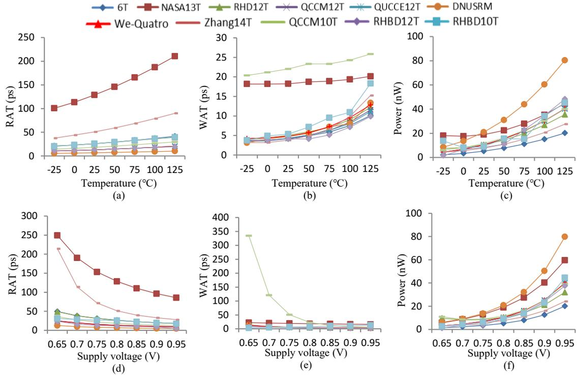
**Fig. 6. Simulation results of VT variation impacts on RAT, WAT, and power for the SRAM designs. (a) Impacts of temperature variations on RAT. (b) Impacts of temperature variations on WAT. (c) Impacts of temperature variations on power. (d) Impacts of supply voltage variations on RAT. (e) Impacts of supply voltage variations on WAT. (f) Impacts of supply voltage variations on power.**
