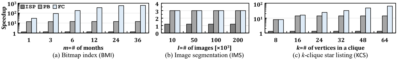
Figure 17: Performance comparison of four computing platforms on three real-world workloads. ISP (In-storage processing), PB (ParaBit), FC (Flash-Cosmos). Speedup values are normalized to OSP (Outside-storage processing). Y-axis is in log-scale.
