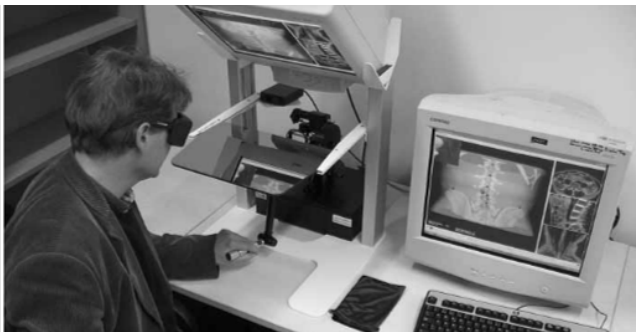
Fig. 2. Virtual lumbar puncture simulator with stereographic visualization [6].
