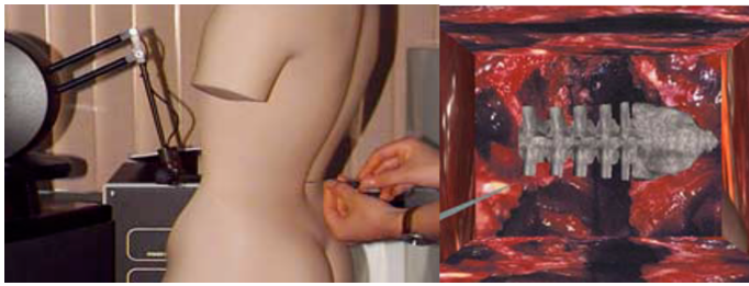
Fig. 1. Haptic device, mannequin, needle and virtual environment of the simulator developed in [13].
