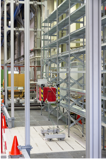
Fig. 4 CABLAR: A fully-constrained CDPR for warehouse logistics. Image source: (Gouttefarde et al 2015b)
