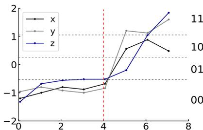
Figure 3: ASAX segmentation with 2 segments
