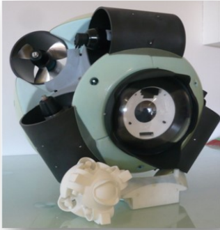
Fig. 1. General view of MEROS underwater vehicle.
