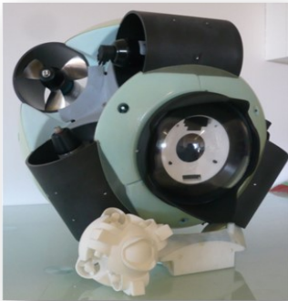
Fig. 1. General view of MEROS underwater vehicle.
