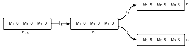
Fig. 4. Trail building in an SGST graph. Two possible trails are valid for the same input values I_v in this example, depending on the order of evaluation of the three status blocks, M_1, M_2, M_3 .
