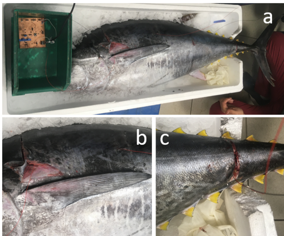
Fig. 5. a) GC communication in a Bluefin Tuna. b) Tx implanted Electrode. c) Rx Implanted Electrode
