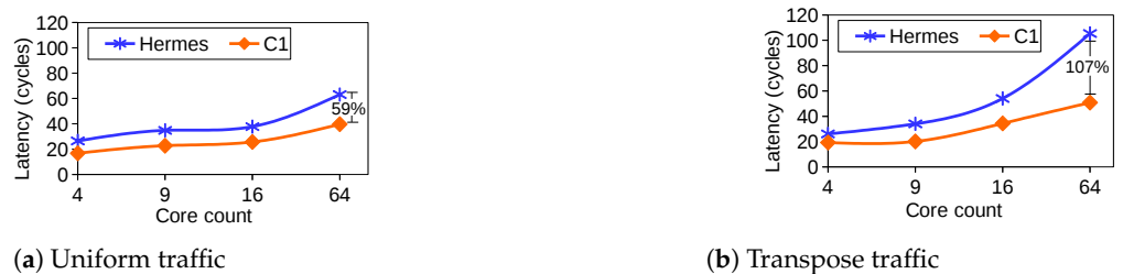
(a) Uniform traffic (b) Transpose traffic Figure 16. Scalability comparison of R-NoC C1 with Hermes [10]. 4: 2 \times 2 mesh; 9: 3 \times 3 mesh, 16: 4 \times 4 mesh, 64: 8 \times 8 mesh network. Latency: average network zero-load latency.
