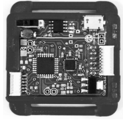
Fig. 1. Developed Wireless Foot Sensor Module.
