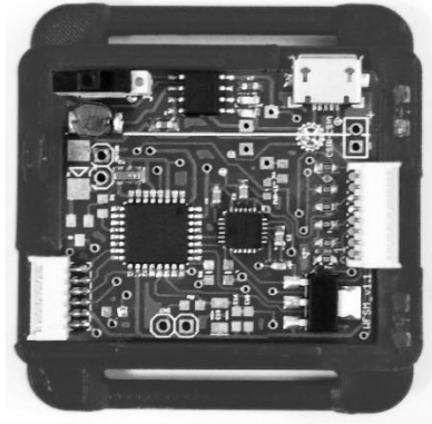
Fig. 1. Developed Wireless Foot Sensor Module.
