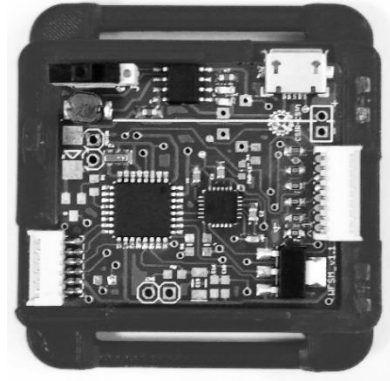
Fig. 1. Developed Wireless Foot Sensor Module.
