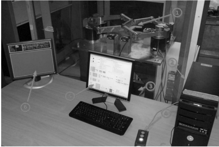
Fig. 7. View of the experimental setup of Dual-V PKM; (1) the mechanical structure of the robot, (2) the host PC, (3) the target PC, (4) emergency stop, (5) host monitor, (6) xPC target monitor.
