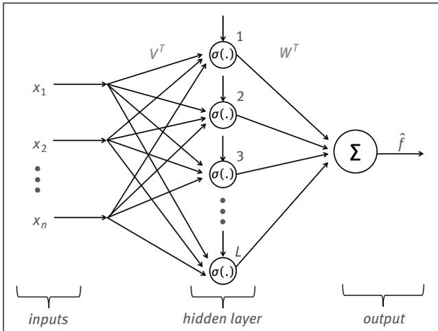
Fig. 4. Schematic view of a three-layer NN.
