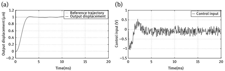
**Fig. 6.** Step response in non disturbed case with RISE-NN controller: (a) Output displacement and (b) Control input.
