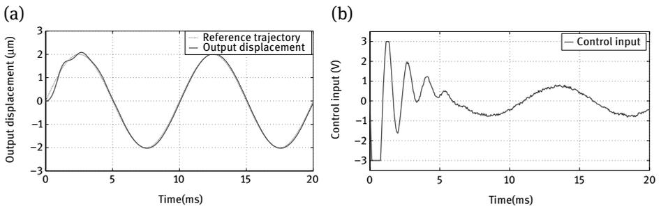
**Fig. 7.** Tracking of a sinusoidal reference trajectory in non disturbed case with PD controller: (a) Output displacement and (b) Control input.
