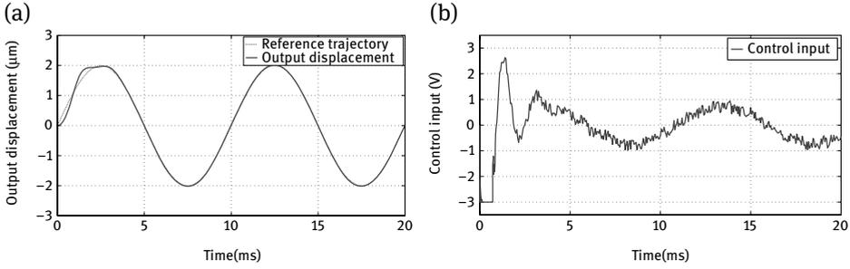
**Fig. 8.** Tracking of a sinusoidal reference trajectory in non disturbed case with RISE-NN controller: (a) Output displacement and (b) Control input.
