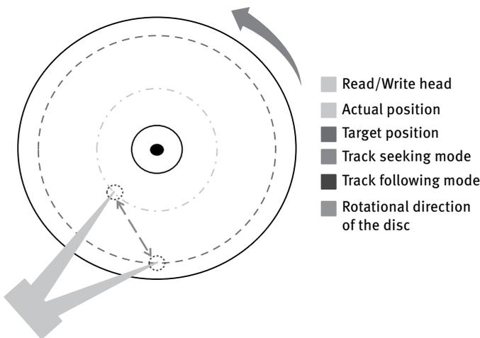
Fig. 2. Illustration of the main operating functions of a HDD servo-system.
