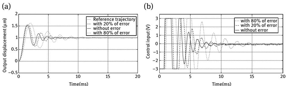
**Fig. 12.** Robustness towards parameters' uncertainties with PD controller: (a) Output displacement and (b) Control input.
