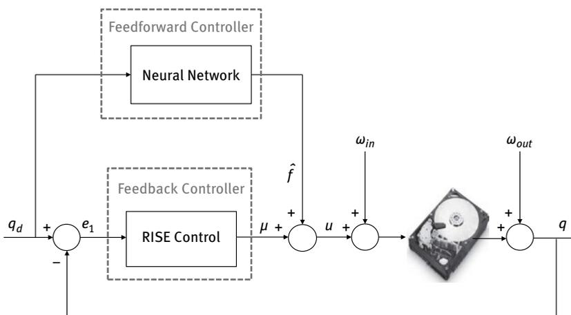
Fig. 3. Overview of the control scheme including a RISE feedback with a NN feedforward.
