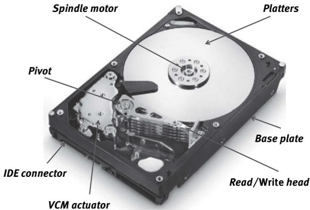
**Fig. 1.** View of the main components of a typical HDD.
