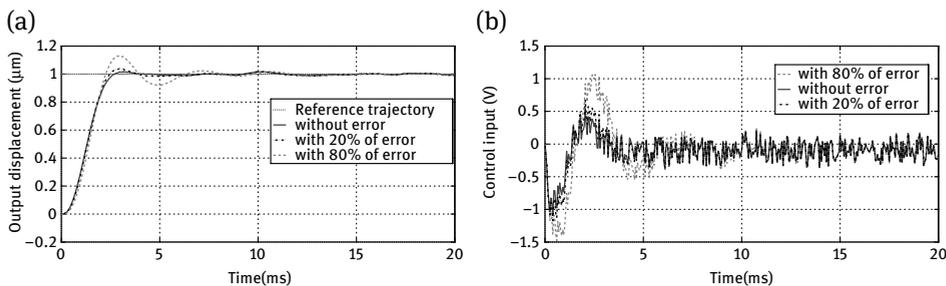
**Fig. 13.** Robustness towards parameters' uncertainties with RISE-NN controller: (a) Output displacement and (b) Control input.
