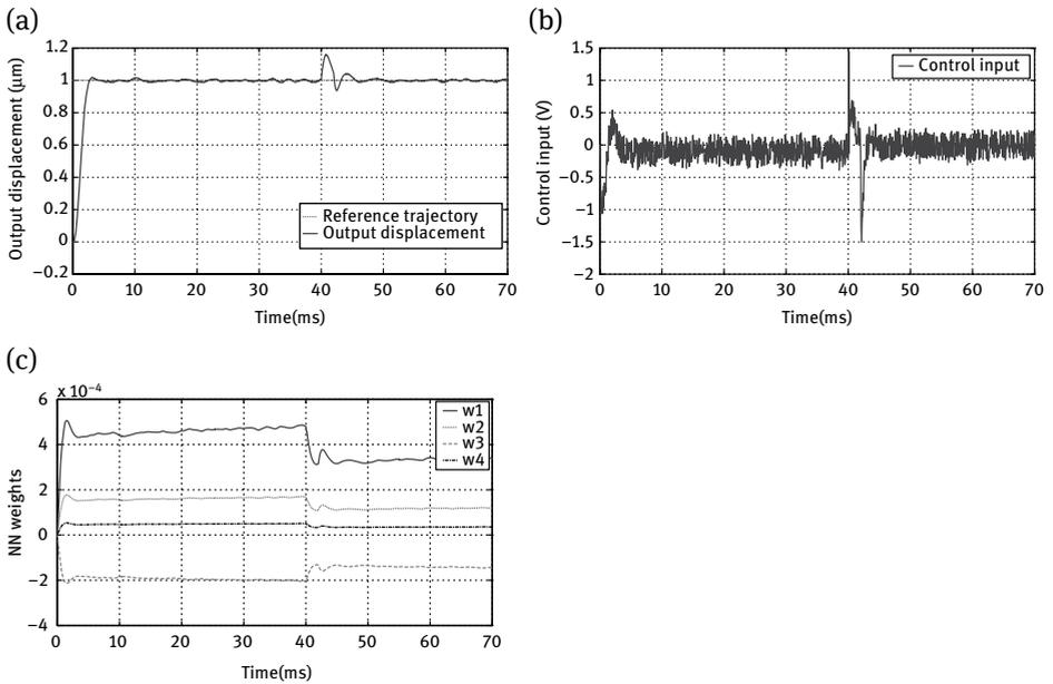
**Fig. 11.** Tracking under external disturbances with RISE-NN controller: (a) Output displacement, (b) Control input, and (c) Time history of the neural network weights.
