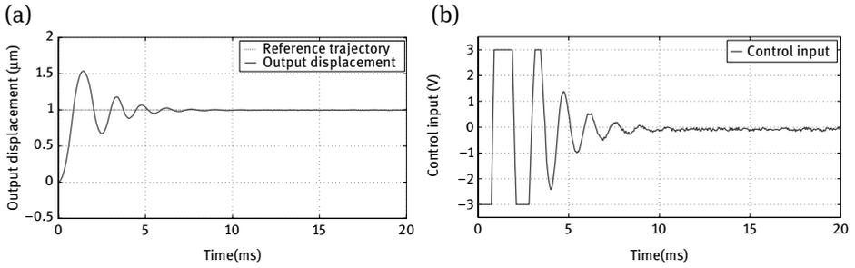
**Fig. 5.** Step response in non disturbed case with PD controller: (a) Output displacement and (b) Control input.
