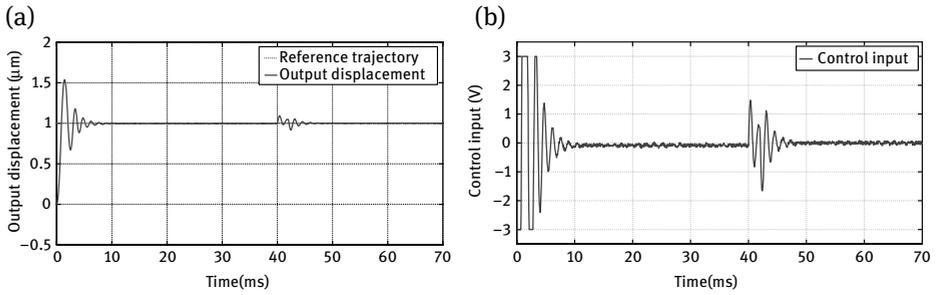
**Fig. 10.** Tracking under external disturbances with PD controller: (a) Output displacement and (b) Control input.
