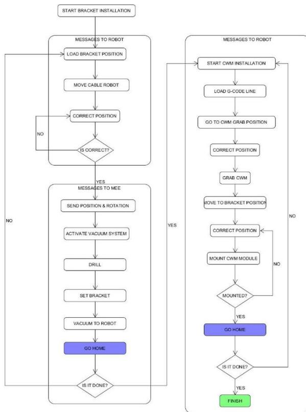
Figure 8: State machine simplified diagram
