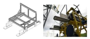
Figure 5: Stabilizer of the robot's frame. Left: CAD. Right: real prototype during the opening of the stabilizers.
