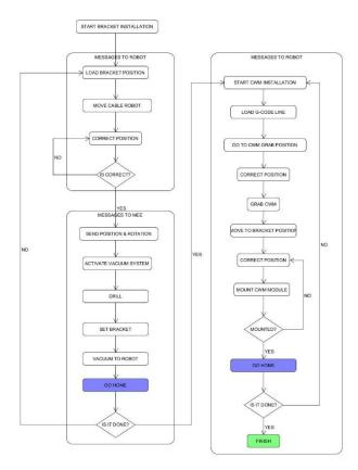
Figure 8: State machine simplified diagram
