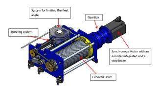
Figure 3: CAD view of the VICINAY Winch WB21.L.30S.1
