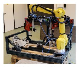
Figure 4: Robotic arm and its tools before mounting on the CDPR platform.
