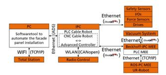
Figure 7: Scheme of the hardware and wiring of the HEPHAESTUS cable robot.
