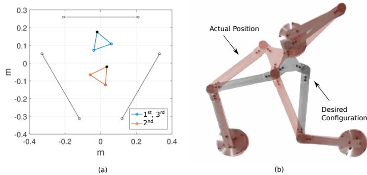
**Fig. 3.** (a) Task to be executed and (b) Actual and desired configurations for the  $3\text{RRR}$
