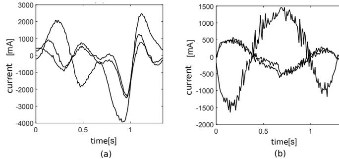
Fig. 5. Currents of the (a) non-redundant and (b) redundant actuators using the Two-Stage Global Strategy
