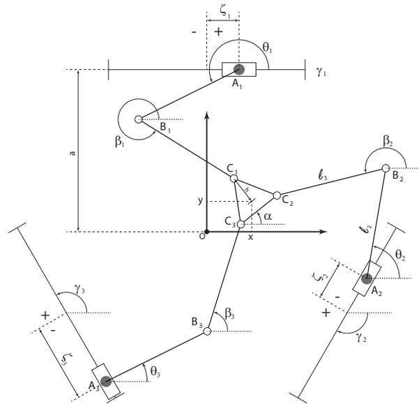
**Fig. 2.** Geometric details of the 3PRRR [10]
