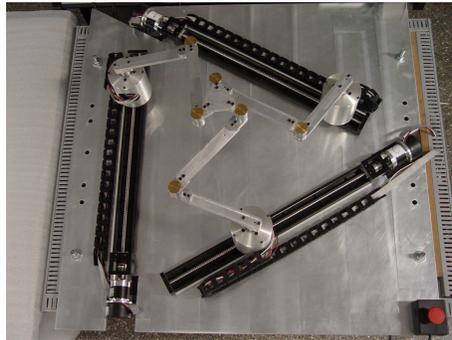
**Fig. 1.** 3PRRR: the kinematically redundant planar parallel manipulator
