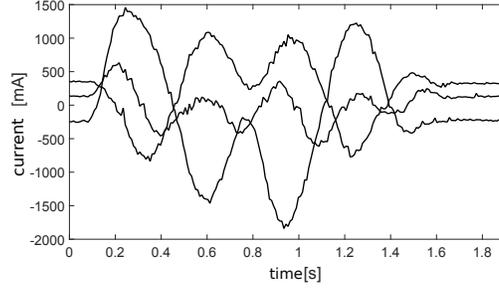
Fig. 4. Non-redundant actuators' currents using the Direct Global Strategy
